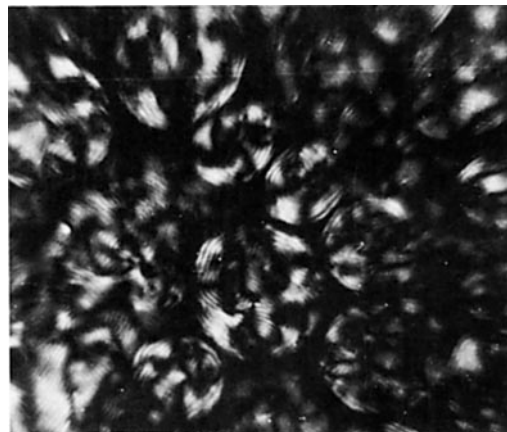
Figure 6 Photomicrograph of THC showing a “fingerprint” texture for the cholesteric liquid crystalline phase at 298 K at 500× magnification.
